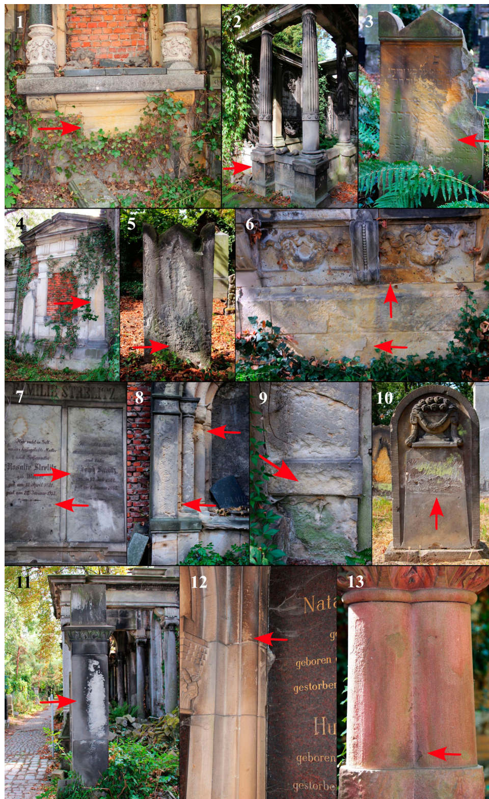
Figure 1. Gravestones at the historical Jewish cemetery in Wrocław (Poland) with traces of biodeterioration. Red arrows mark sampling locations.
